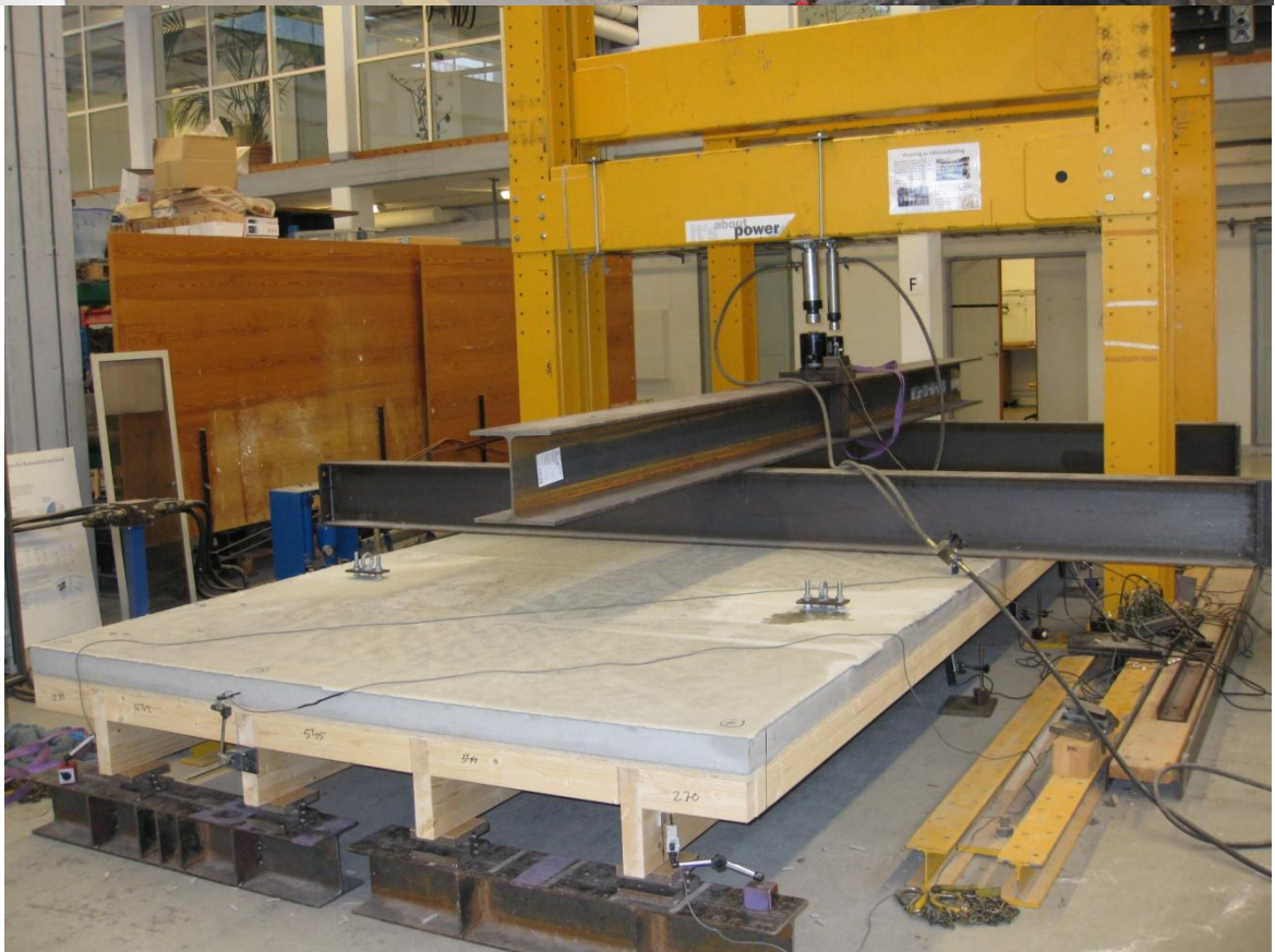
Figure 4.5 Top: Rig used for testing of the floor using SFS-screw connectors. Bottom: Rig used for testing of the floor using the plug-type connection
