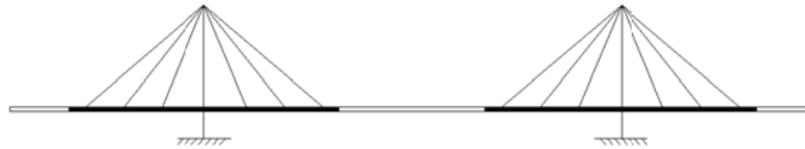
Figure 4-19: Self anchored system.
