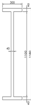
Figure 4-15: Determined size of the main girders.
