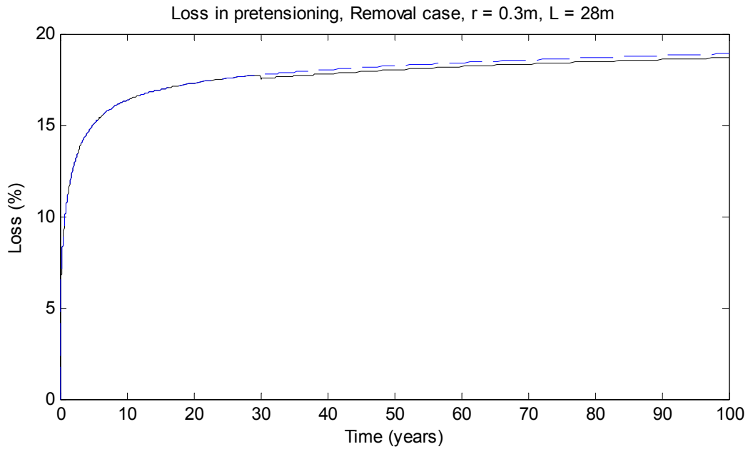
Figure 8-24: Prestressing loss with elastic effects included for bridge with span-length L = 20\text{m} , when 300 mm is removed from each flange. The dashed line is the corresponding loss in prestress from the reference calculation.
