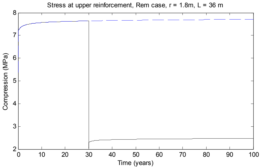
Figure 8-15: Compression at upper reinforcement level as a function of time for span-length L = 36\text{m} , when 1800\text{ mm} is removed from each flange (entire flange). The dashed line is the corresponding stress from the reference calculation.
