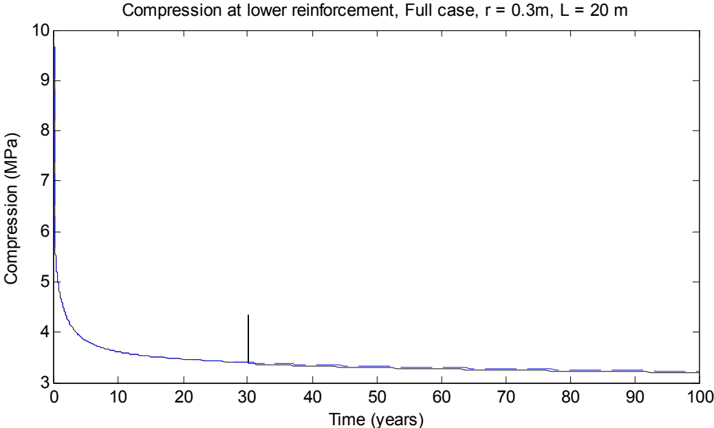
Figure 8-34: Compression at lower reinforcement level as a function of time for span-length L = 20\text{m} , when 300 mm is removed and replaced from each flange. The dashed line is the corresponding stress from the reference calculation.
