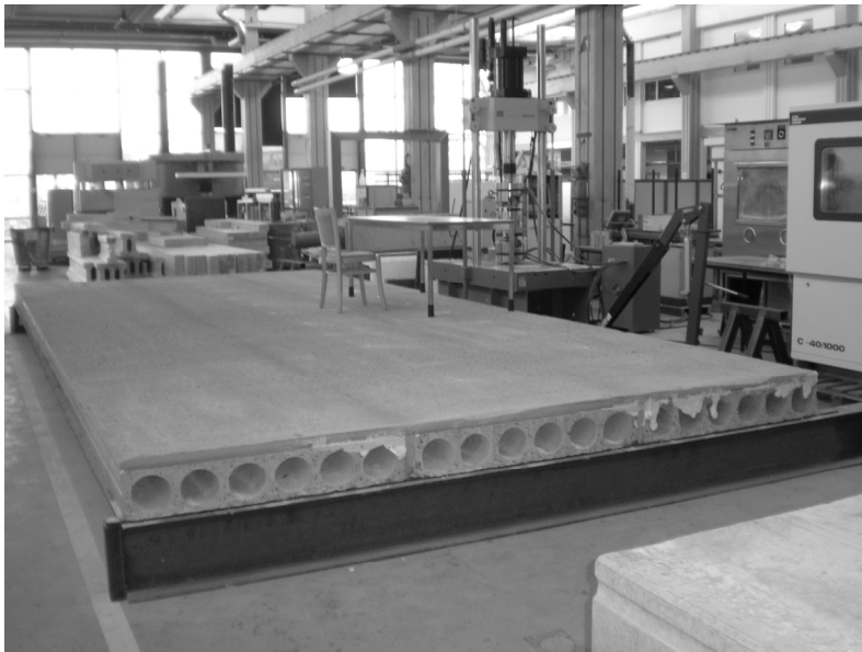
Figure 7.1. Experimental floor structure.
