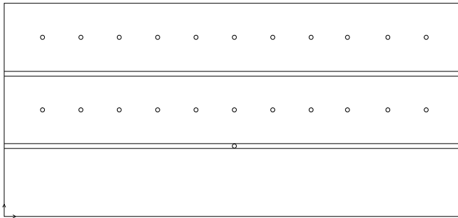
Figure 7.2. Measurement set up. The figure shows where the accelerometers were placed.
