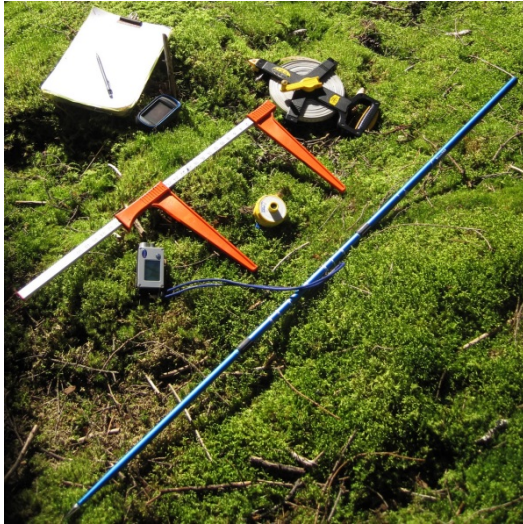
Figure 3. Fieldwork equipment: calipers, GPS unit, hypsometer, transponder, measuring tape, measuring stick and field log (photo taken during fieldwork).
