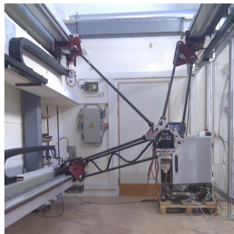
Figure 1: Gantry-Tau robot denoted L2.
