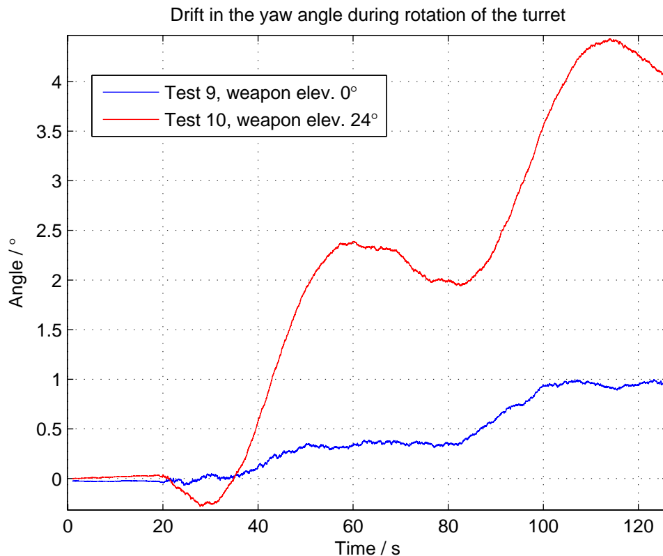
Figure 9.2: Two tests where the turret performed two full rotations with the weapon at different elevation angles. A loss in heading estimate accuracy was observed when the weapon elevation angle was significantly different from the original 0° position.
