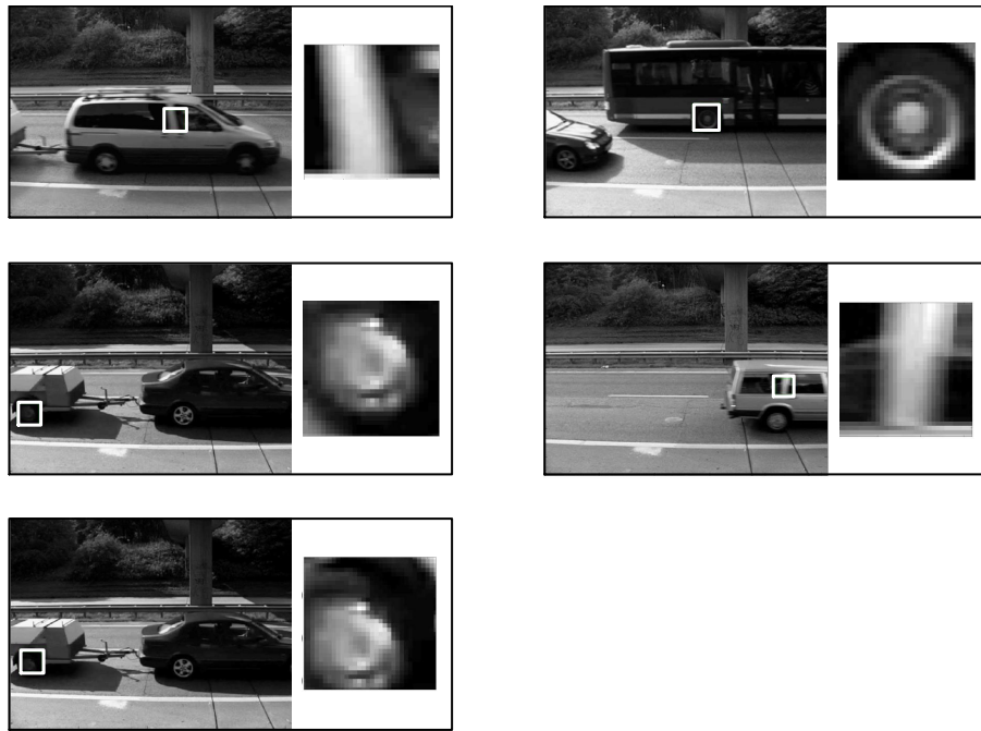
Figure 5.3: Out of 100,000 randomly sampled negative windows, only 28 false positive windows pass the cascade classification, where 23 of those are actually near hits on car wheels. The five remaining false positive windows are illustrated in the figure above. Out of these, there are three windows that belong to another vehicle type and could therefore also be considered a near hit of a wheel. As a result, there is merely two false positive windows of the total 100,000 negative windows that are truly misclassified in the cascade classification.
