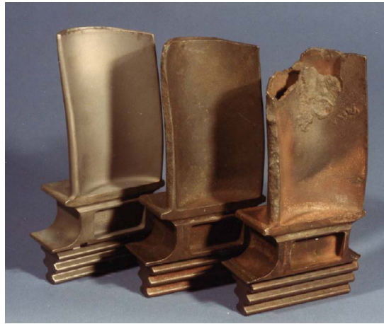
Figure 4.7: Sulfidation failure on a 1970's low-firing temperature machine [78]
