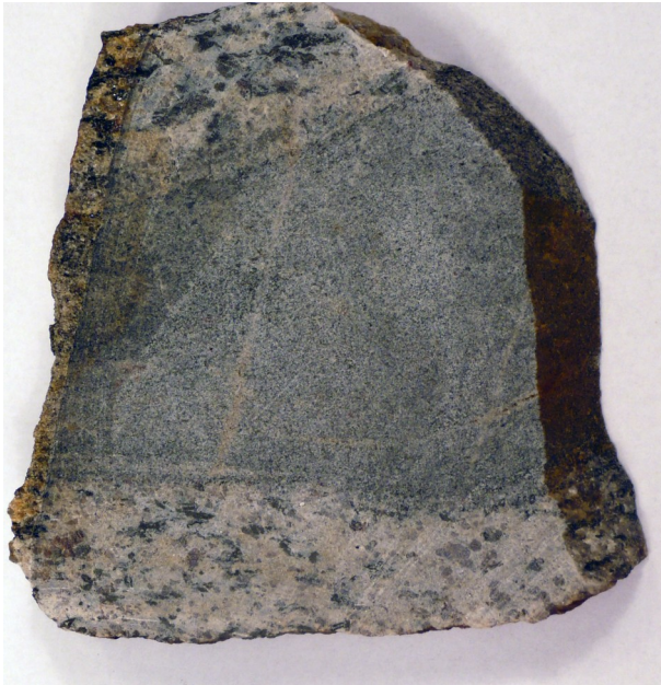
Fig. 9. Fine to medium-grained grey gneiss from Romeleklint with a darker fine-grained band (JU25A).
