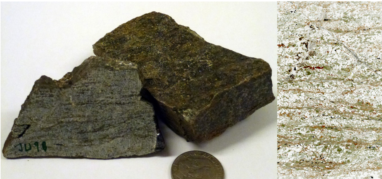
Fig. 27. Amphibolite from Romeklint (JU9B) with thin section to the right (width 20 mm).
