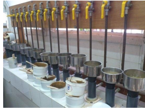
Figure 5.16. The extraction of soil salinity extract using vacuum.
