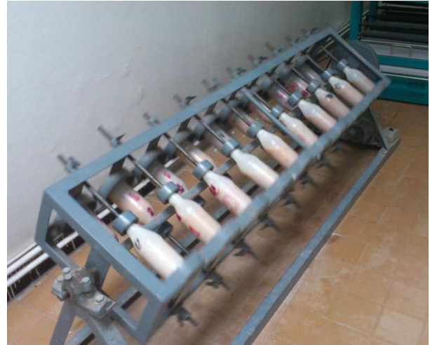
Figure 5.18. Agitation of soil samples to prepare pipette-Robinson analysis.
