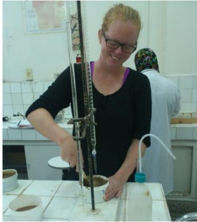
Figure 5.15. The preparation of the soil salinity extract paste.
