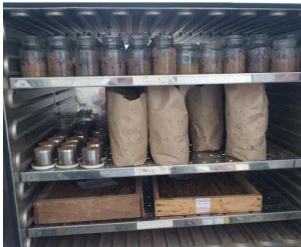
Figure 5.13. Soil samples being dried in an oven.
