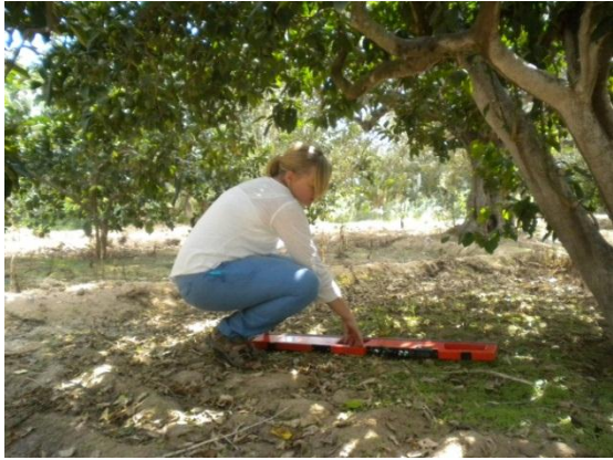
Figure 5.7. EM38 measurements being taken.
