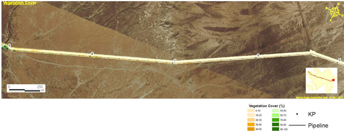
Figure 3.24: Calculated Vegetation Cover spatial grid 2007 from NDVI spatial grid 2007 for sample area 1 (Backdrop – IKONOS image).
