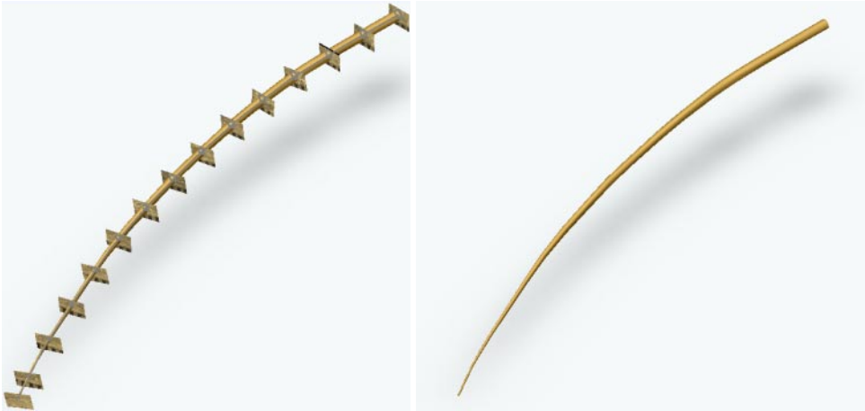
Figure 4.3: The three-dimensional geometry model created from micrographs of cross-sections. The cross-sections are indicated to the left and the final geometry to the right.
