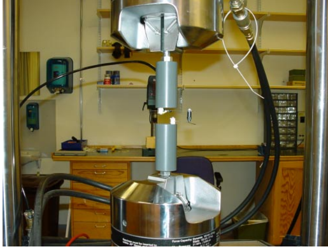
Figure 3.1: Bending stiffness test equipment mounted in an MTS-testing machine.
