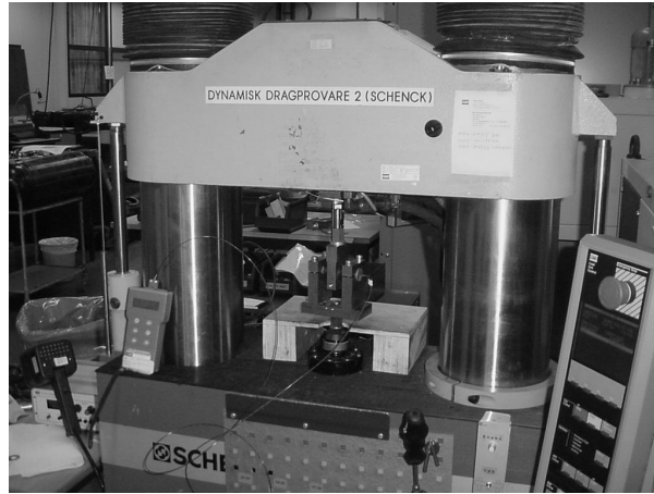
Figure 3.1: The machine used for testing. A Schenck static/dynamic tensile testing machine [3].
