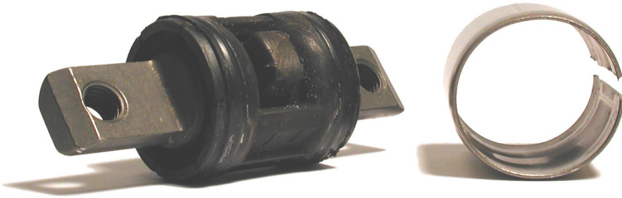
Figure 2.2: The hydrobushing parts. Interior and cover.
