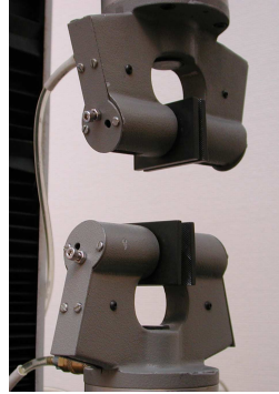
Figure 4.1: The Instron 4200 / 4300 / 4400, tensile testing machine
