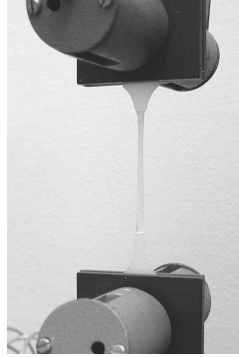
Figure 4.4: Tensile testing of the MILK material
