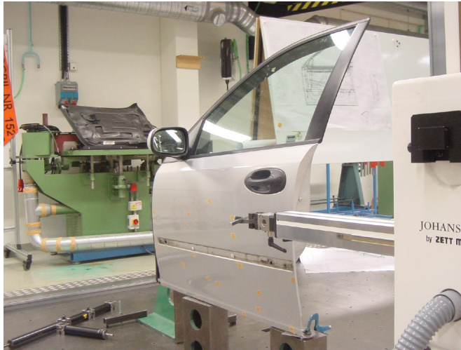
Figure 6.1 Position measurement system used to determine the response locations.
