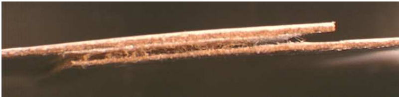
Figure 3.13: Fracture propagation in the lower laminate
