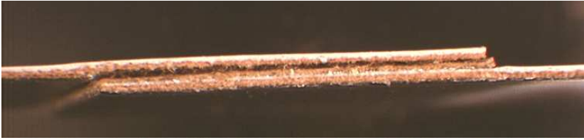
Figure 3.12: Fracture propagation in the upper laminate
