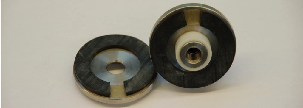
Figure 3-20 Cut out of the EPDM to make room for the strain gauges
