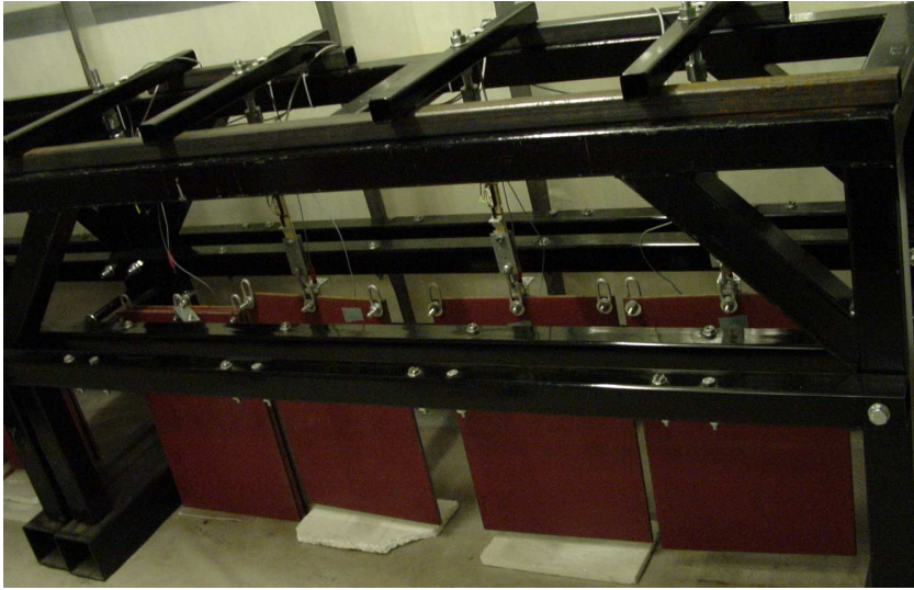
Figure 3.8: Test rig used for creep tests.
