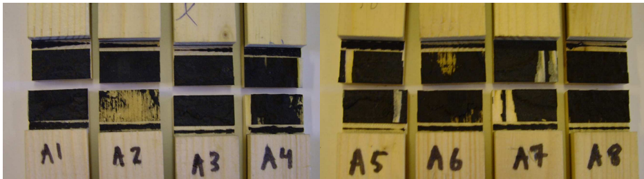
Figure 3.7: Failure types of the test specimens.
