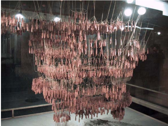
A funicular model of Sagrada Familia
