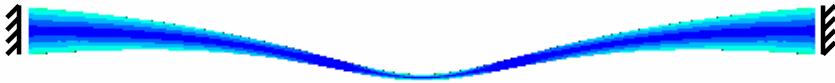
Fixed beam. The largest heights (12m) are in the ends and it is smallest (1.6m) in the middle. Maximum deformation is 0.6m, and maximum field stress is 23 MPa
