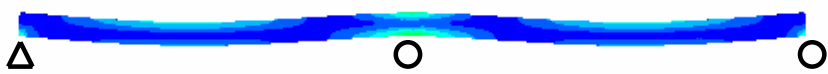
Roller supported beam. Maximum deformation is 0.12m, and maximum field stress is 14MPa
