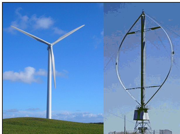
Figure 2.1: Left: Horizontal axis wind turbine [B] Right: Vertical axis wind turbine [C]
