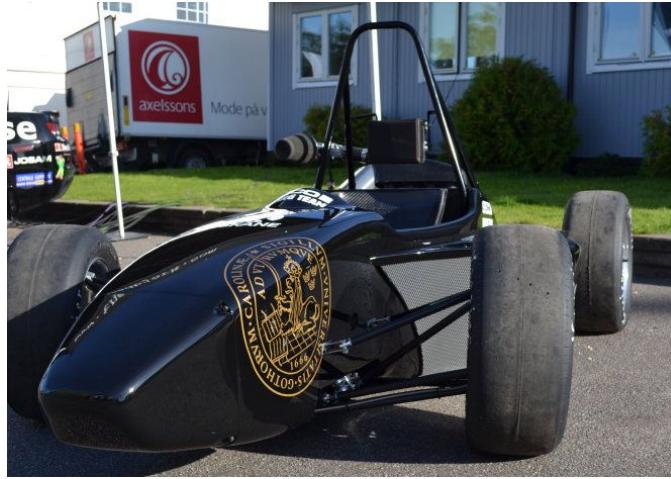
Figure 1.4: A double wishbone suspension is used in many competitive race-cars such as this Formula Student [4] car LUR5 from LU Racing [5].
