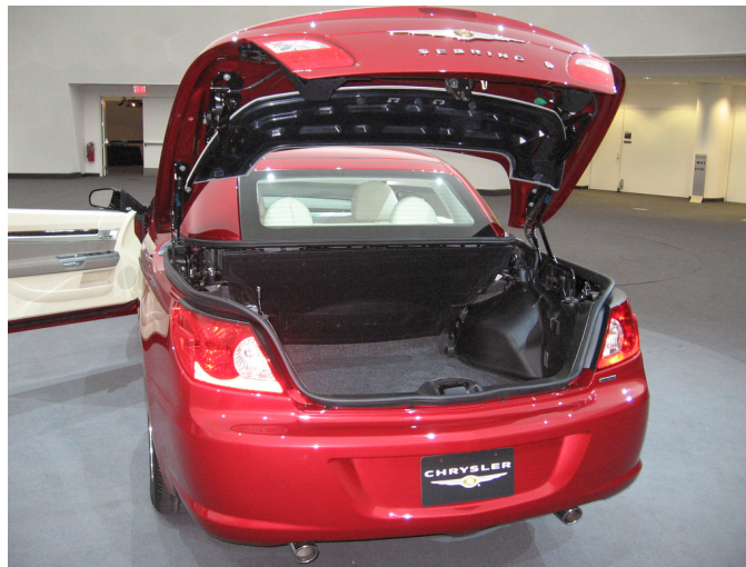
Figure 1.5: Chrysler Sebring 2005 has a four-bar linkage to support the trunk cover motion.
