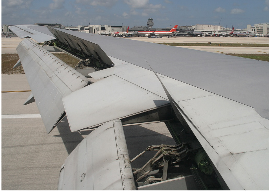
Figure 1.1: The flaps of an airplane changes the aerodynamic property of a wing to allow start, landing and altitude changes. Photograph by Jerome Mervelet [1]
