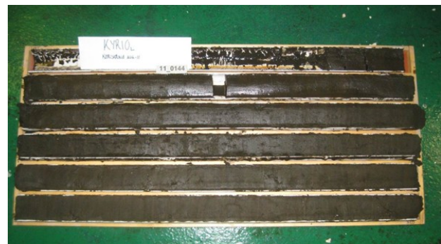
Figure 8: Photo of Karlskrona core showing the brownish homogeneous gyttja.
