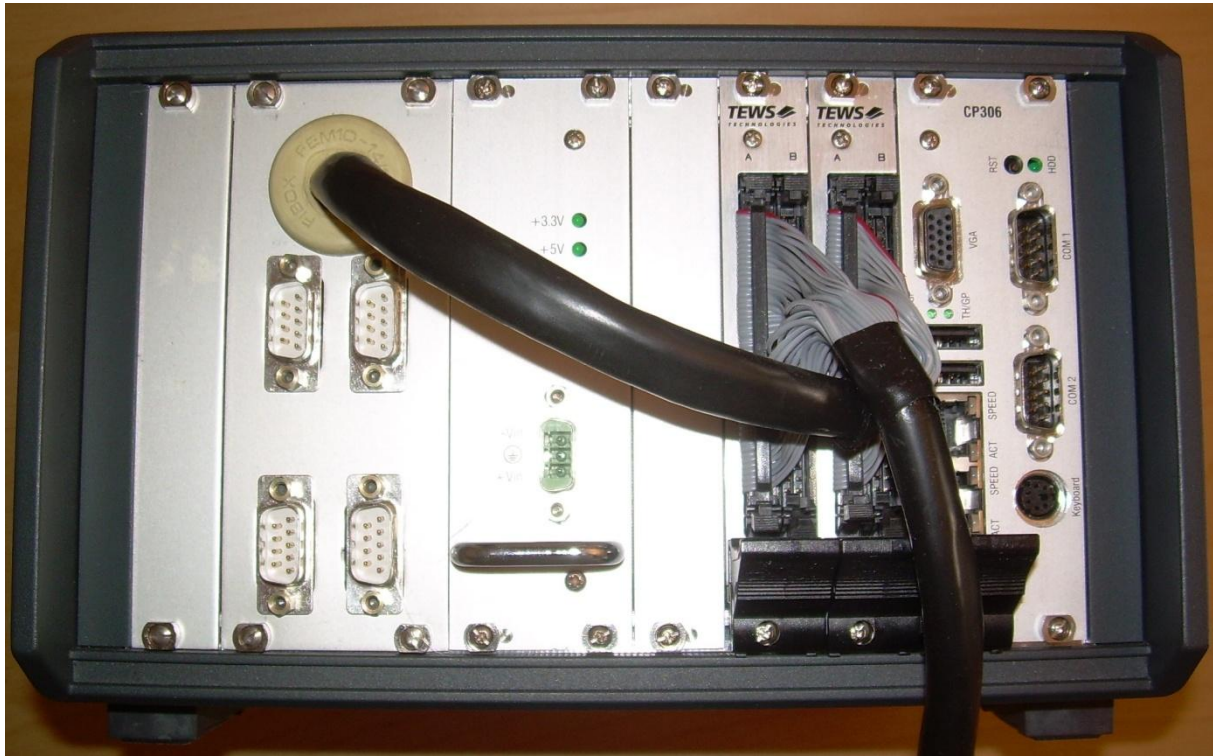
Figure 1. Industrial PC box for Motionlogger 2. To the left is the connector plate for the encoder sensor. Next to the connector plate is the power supply. Located next to the power supply is connectors for TIP logging cards. And to the right is the computer itself.
