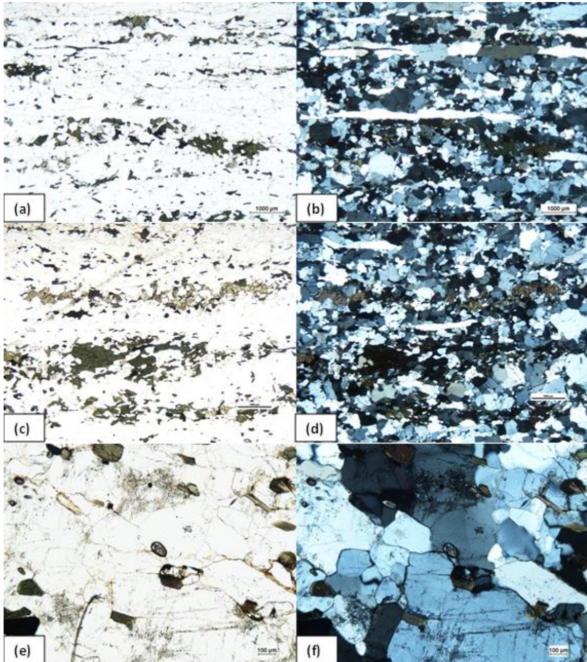
Fig. 15. (a)-(f) Photomicrographs of mylonitic gneiss, sample NMA11052a. (a) PPL, Dark and light bands composed of different proportions of plagioclase, hornblende and biotite and conspicuous quartz ribbons. (b) CPL, same view as in a. (c) PPL, Plagioclase, quartz, hornblende and biotite. Hornblende is brown-green pleochroic. (d) CPL, same view as in c. (e) PPL, Granoblastic plagioclase with local saussuritization. Small zircon grain in the center of the photo. (f) CPL, same view as in e.
