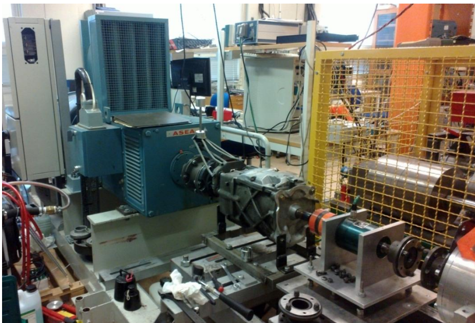
Figure 2 - Traditional test bench. From left; big braking motor, gearbox, torque sensor and in the rear corner the tested machine
