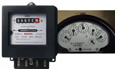
Figure 16: Example of electromechanical meters [23]
