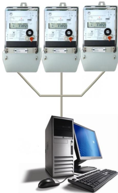
Figure 60: Communication with three meters by RS232
