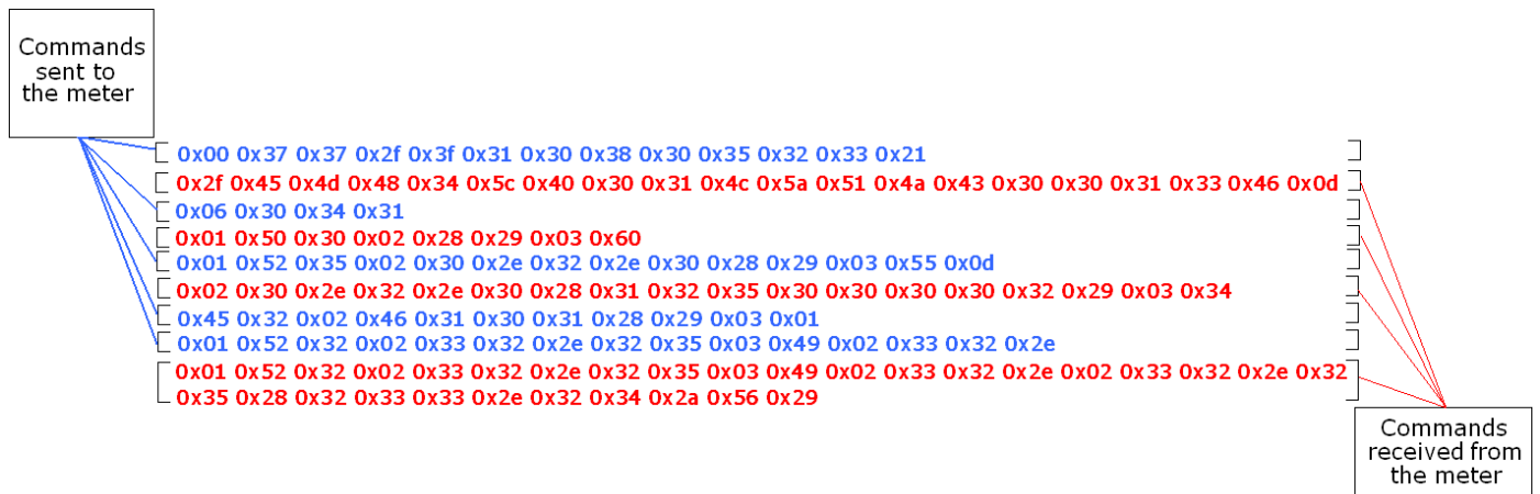
Figure 55: Communication protocol to receive the value of the voltage at line 1
