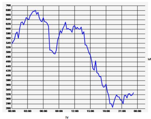
Figure 9: Example of a graphic where it is shown the intermittence of wind power signal during a day. [27]
