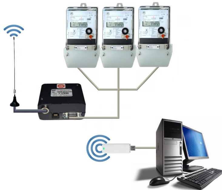
Figure 63: Communication with three meters by GSM
