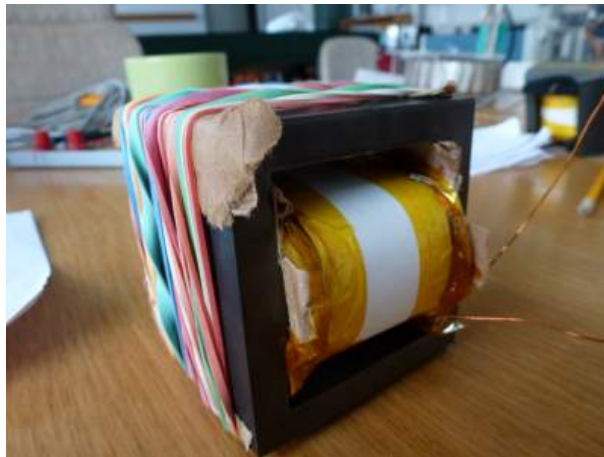
Figure C.1: The resonance inductance
