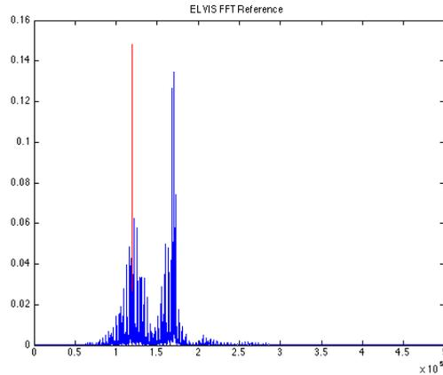
Figure 12: As apparent in the picture, even if the transmitted signal is mainly 170 kHz, there is a significant contribution from a 118 kHz signal.
