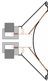
Figure 2: When pressure changes around the diaphragm, the coils will move and the magnetic field will be submitted to change.
