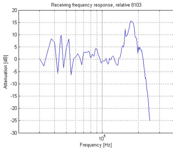
Hydrophone 1 was measured every 2,5 kHz from 30-250 kHz plus an additional recording at 45,5 kHz.
