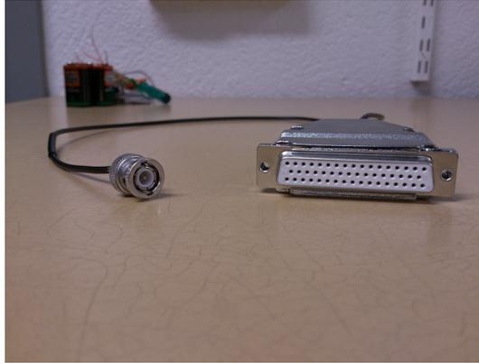
Figure 5: The home made adaptor, BNC to D-sub50.
