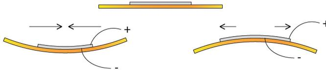
Figure 1: The principle on how piezoresistive material changes its length and therefore resistance.
