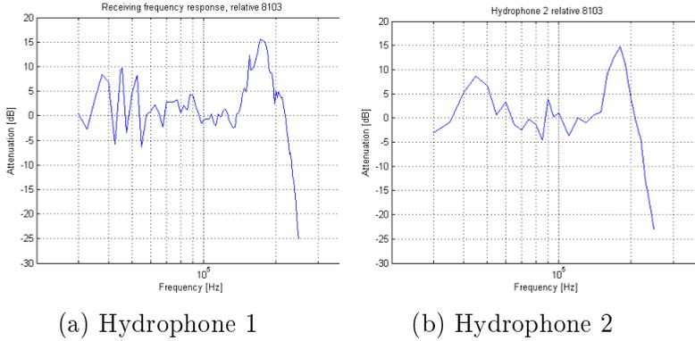
Figure 18: The plots show the comparing response for the respective hydrophones
