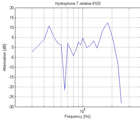
Large peak at 45 kHz but extreme attenuation at 65 kHz.
