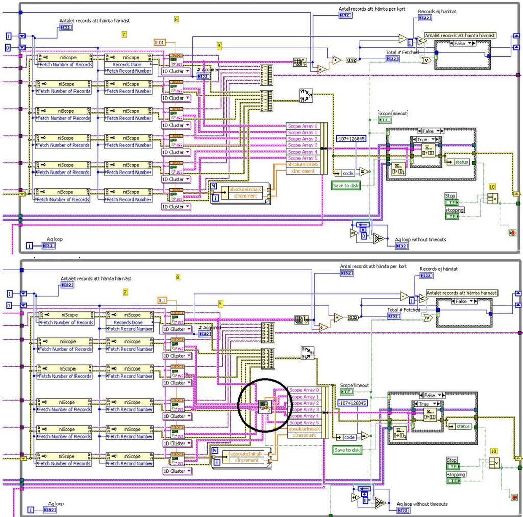
Figure 8: The upper picture shows the ELVIS acquisition loop before modification, the lower one after. As apparent, it is only a minor modification
