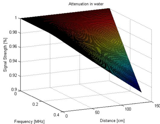
Figure 14: The graph shows the attenuation in water depending on distance and frequency. The graph ranges from 0-150 cm and 0-0.4 MHz
