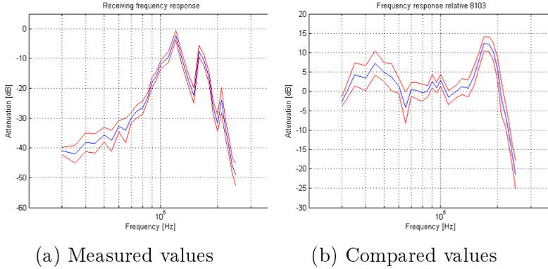
Figure 20: This figure shows the standard deviation instead of the maximum and minimum values.
