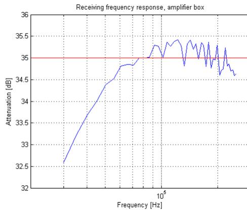
Figure 15: The frequency response from the amplifier. The red line shows the theoretical amplification of 35 dB.
