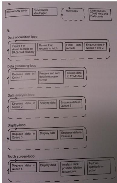
Figure 3: A flow chart that explains how ELVIS works, the loops run independently.
