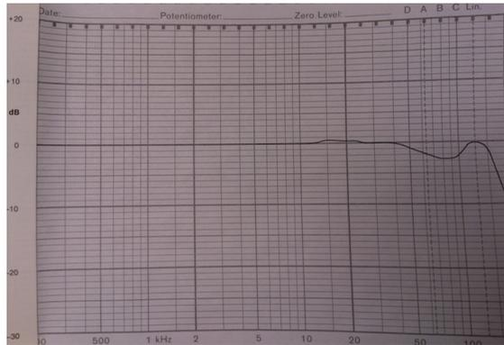
Figure 21: The calibration graph that was delivered together with 8103. 0 in this graph is normalized around  $-211.3 \text{ dB re } 1\text{V}/\mu\text{Pa}$  or  $27.2 \mu\text{V}/\text{Pa}$ .
