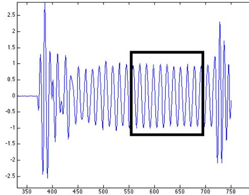
Figure 13: The figure shows the general appearance of a single pulse. The black square shows the area of interest. The large spikes in the beginning and the end are due to the 118 kHz excitation pulses from the projector.
