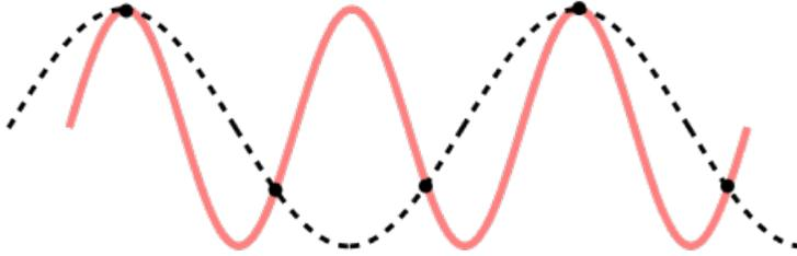
Figure 4: With too low sample rate, a higher frequency sinusoid can appear as a lower frequency.
