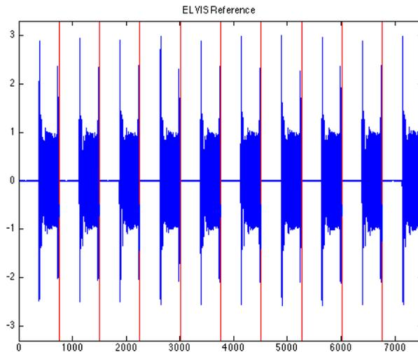
Figure 11: The red lines indicate a start of each pulse. The flat area is the pre-trig recording.
