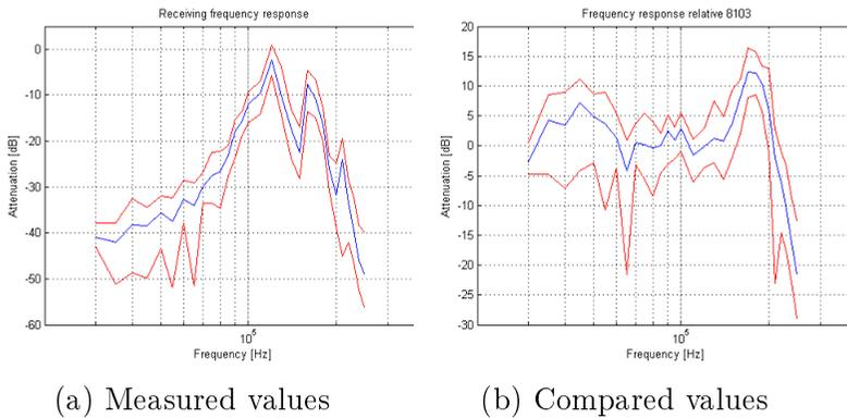
Figure 19: The red lines show the minimum and maximum value from all hydrophones, the blue line is the average value.
