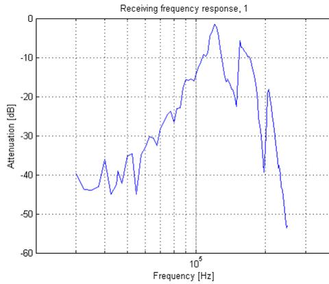
Figure 16: The plot shows the frequency response for hydrophone 1.
