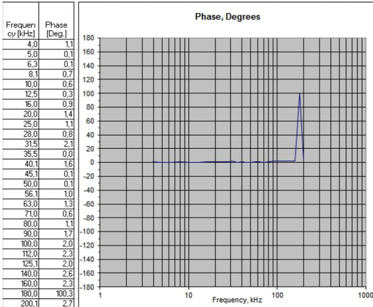
Figure 25: Brüel & Kjær’s result when measuring the phase response. This was given to us in their pre-study but excluded from their final results.
