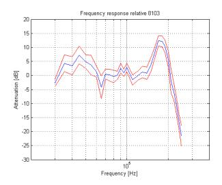
The conclusion is that they perform very well compared to each other. There are two resonances present, one around 45 kHz and one at 170 kHz. After 200 kHz the performance drops drastically and around 65 kHz there is a slight performance drop as well. This method demands a lot from the reference and this is the largest error in our results and therefore no absolute results can be presented.
