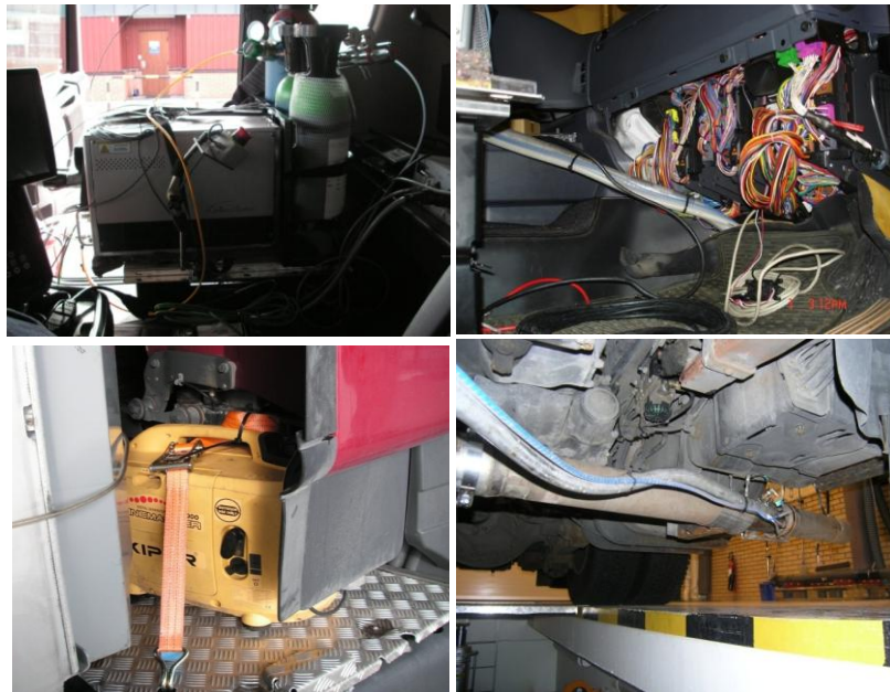
Figure 19 Mounting of PEMS inside cabin
