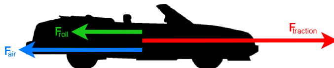
Figure 3.2: Basic forces acting on a rolling car
