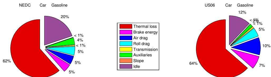
Figure 3.9: Chemical energy distribution required in the NEDC (left) and US06 (right) drive cycle.
