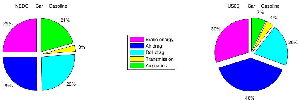
Figure 3.7: Mechanical energy distribution required in NEDC (left) and US06 (right) drive cycles.
