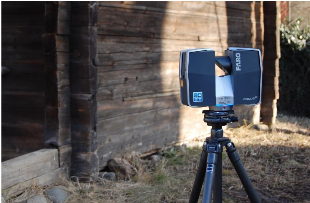
Figure 7. Faro Focus 3D scanner on the field. (Picture: Linda Nesi, 2013).
