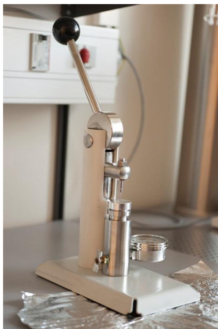
Figure 11. The sample pressing device, manufactured by National Electrostatics Corp.
