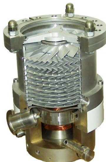
Figure 6. A cut-through of a turbomolecular pump, showing the opposite inclinations of the rotor and stator blades. Figure obtained from
