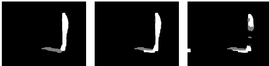
(a) Training result using only intensity. (b) Training result using intensity and chromaticity. (c) Training result using intensity, chromaticity and texture.
