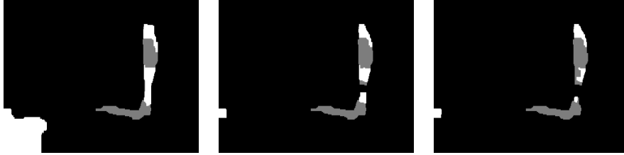
(a) Segmentation using weights designed for intensity. (b) Segmentation using weights designed for intensity and chromaticity. (c) Segmentation using weights designed for intensity, chromaticity and texture.
