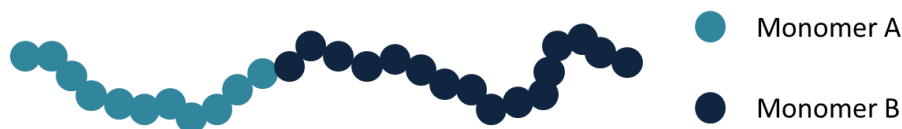
Figure 2. The structure of a di-block copolymer. The two monomer types form distinct polymer chains connected at the ends.
