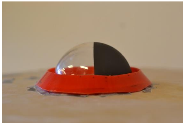
Figure 6-3 Modified channel jet prototype to achieve air cushion mechanism
