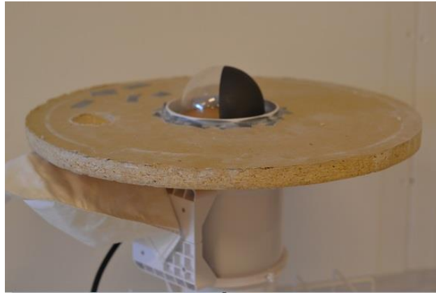
Figure 6-2 Channel jet prototype with dust chamber suspension
