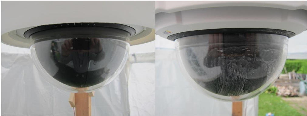
Figure 9-2 Protected dome (left) and unprotected reference dome (right)
