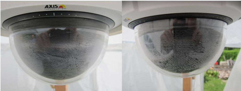
Figure 9-4 Protected dome (left) and unprotected reference dome (right)
