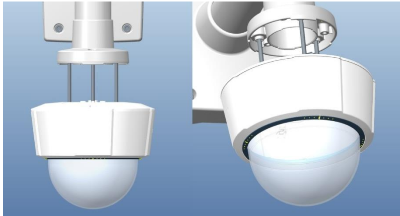
Figure 10-2 Standoff screws between camera housing and bracket
