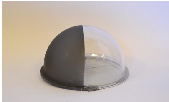
Figure 6-1 Test dome halfway coated with graphite spray
