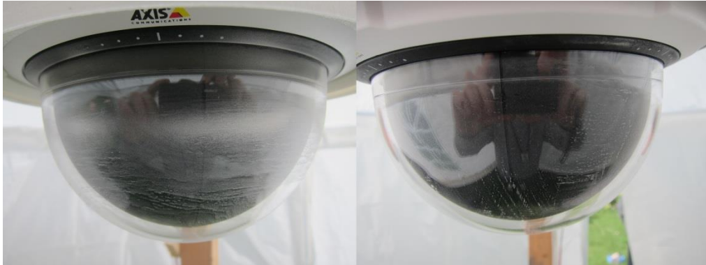
Figure 9-3 Protected dome (left) and unprotected reference dome (right)
