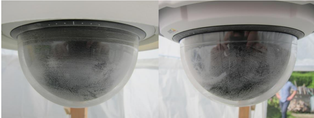
Figure 9-6 Protected dome (left) and unprotected reference dome (right)
