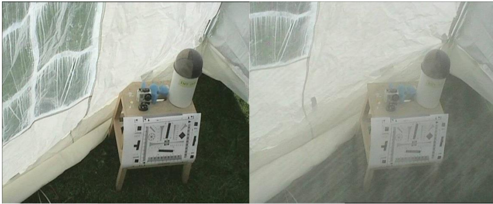
Figure 9-8 Picture from unprotected reference before (left) and after (right) contamination
