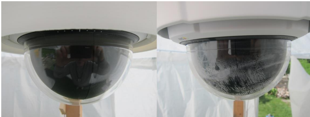
Figure 9-1 Protected dome (left) and unprotected reference dome (right)
