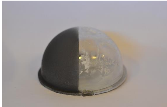
Figure 6-8 Contaminated reference dome
