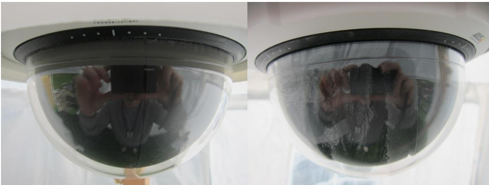
Figure 9-5 Protected dome with antistatic coating (left) and antistatic coated reference dome (right)
