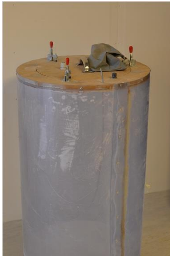
Figure 6-7 Dust test chamber with inlet, filtered outlet and suspension lid
