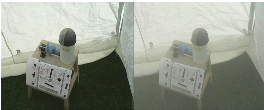
Figure 9-7 Picture from protected camera before (left) and after (right) contamination The picture taken after grinding the concrete slab, although displaying a grey shade as the surrounding air was not entirely cleared, did not contain any stains or deviations.
