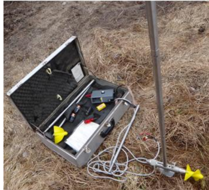
Figure 12 Velocitymeter used. Sendra Díaz and Österlöf, 2013
