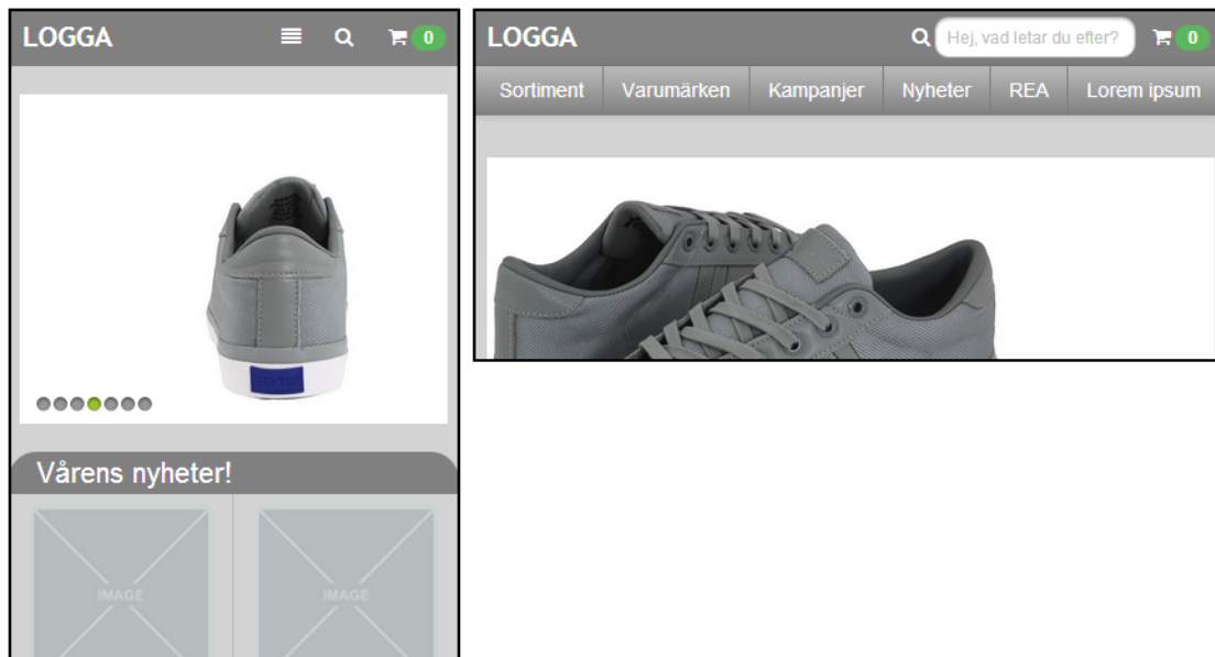
Figure 3.15: Prototype 1 and 2 becomes prototype 6 and 7 when switching from portrait to landscape mode.
