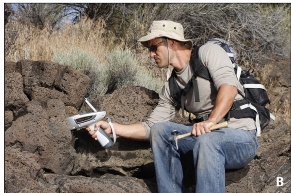
Fig. 1. a. Stationary XRF device, taking up an entire room. Modified after Smithsonian National museum of Natural History (2013; http://mineralsciences.si.edu/facilities/xrf.htm ). b. Portable XRF device. Modified after Thermo Fisher Scientific (2013; http://www.portableas.com/index.php/products/niton-xl3t-950-goldd/ ).
