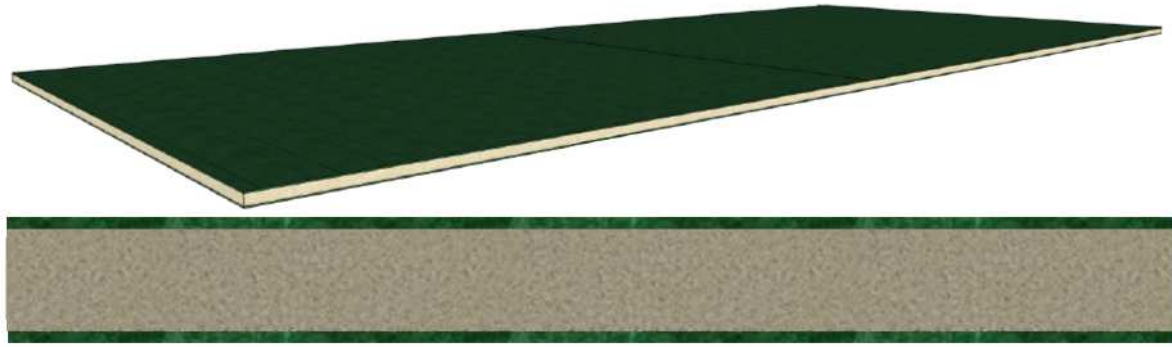
Figure 1. Illustration of an FRP Composite with its laminates on each side of a lightweight core (Evegren, 2010).
