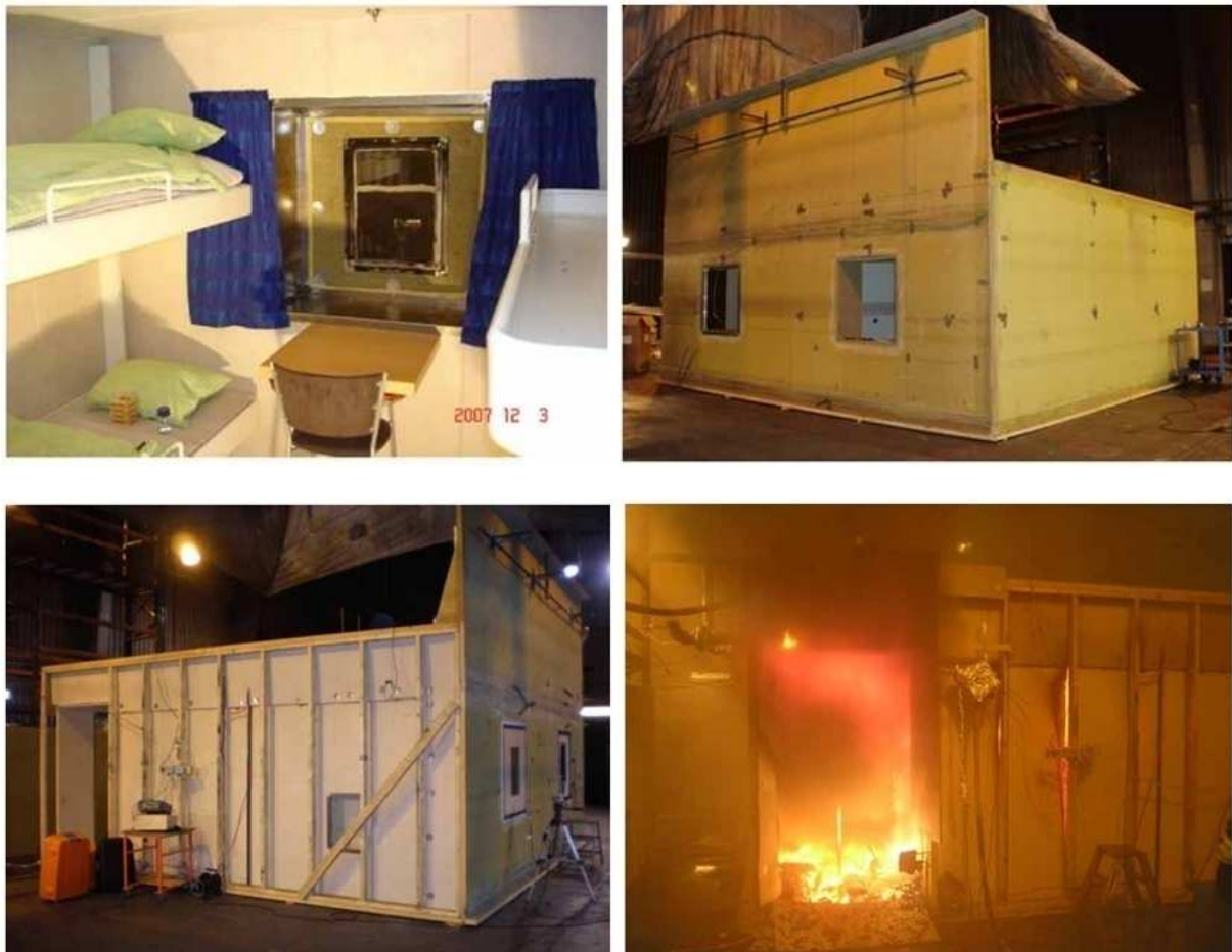
Figure 14. Interior and exterior of the large scale cabin test, before testing commenced. The bottom right image was taken after flashover had occurred in the cabin. Not shown in the interior picture are the luggage and clothes (Hertzberg, Axelsson, & Arvidson, 2008).
