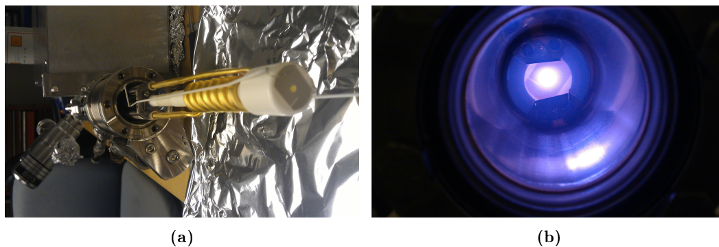
Figure 14: An SVT associates RF 2.75 [23] plasma source lies disassembled in (a), revealing the thick copper coil where the RF signal is passed through during operation. When the plasma is ignited, a distinct glow will be emitted from within the source, as can be seen in (b). The color of the glow depends on the gas, whereat argon (Ar) was used during testing of the plasma source.
