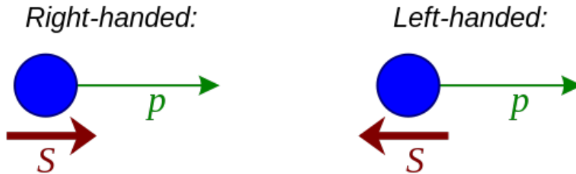
Figure 2: Helicity of a fermion: if the spin and momentum of a fermion are co-directed, the particle is right-handed; if the spin and momentum of a fermion are counter-directed, the particle is left-handed [4]
