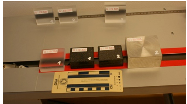
Figure 7. Photograph showing the set up during calibration performed before and after the measurement. The calibration here is using two sets of standards positioned over the measuring track visualized in figure 5. Photo: T. Andolfsson.
