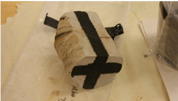
Figure 6. Photo of a drill core sample prepared for measurement in the Thermal Conductivity Scanner. The surfaces which are to be analyzed are planar cut and painted black. Photo: T. Andolfsson.
