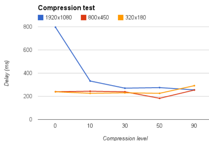
Figure 4.2 Video delay results from tests different levels of compression combined with three different resolutions. Testing was done with VLC according to the test method described in Appendix B using MJPG as video codec.
