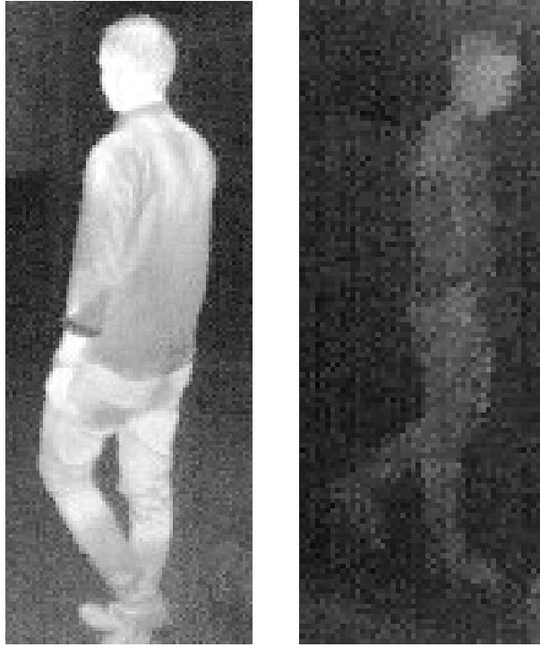
Figure 18: IR images of a human (left) and a reflection of a human (right)
