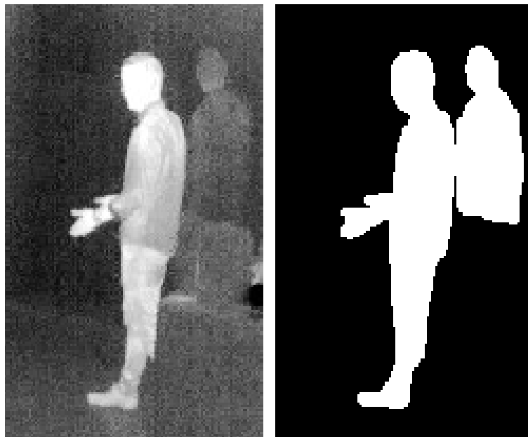
Figure 19: The left image shows when a person is concatenated with his reflection and the right is the corresponding IR segmentation
