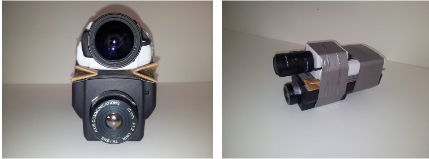
Figure 9: The cameras that were used, the upper white one being the visual camera and the lower black one being the IR camera.
