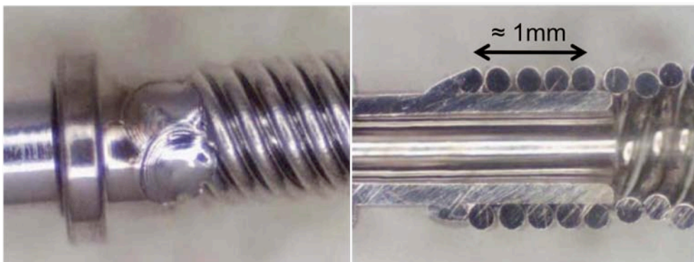
Figure 1.1: Typical join of wire and tube in laser micro welding (according to [SAARECHIEV & JIE 2004A]).
