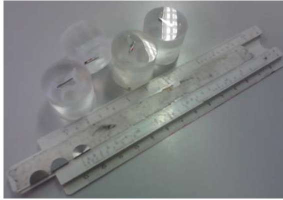
Figure 6.5: Positioning of halved samples on slide rule and embedded samples after producing metallographic cross sections.
