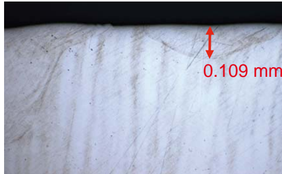
Figure 6.6: Measuring of the welding depth from metallographic sections. Left: weld from a 800 W pulse at 1.3 J, Right: 350 W at 1.3 J.
