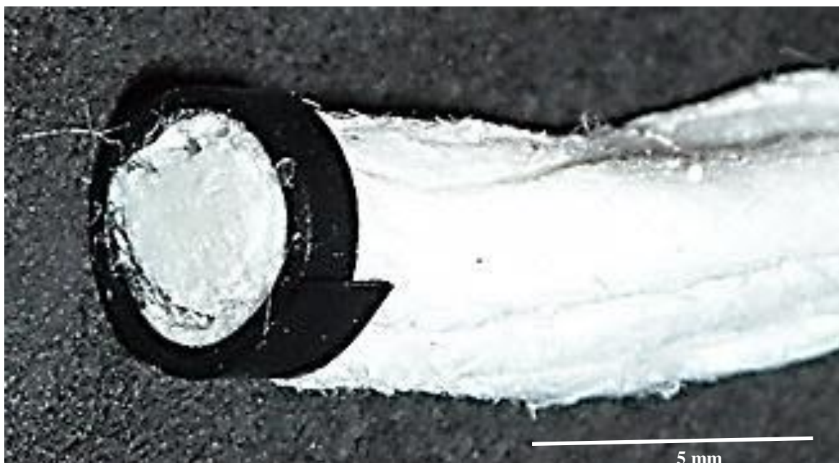
Fig.40E. 3D structure of high porosity aligned PLLA hollow fibers was developed during this master work.
