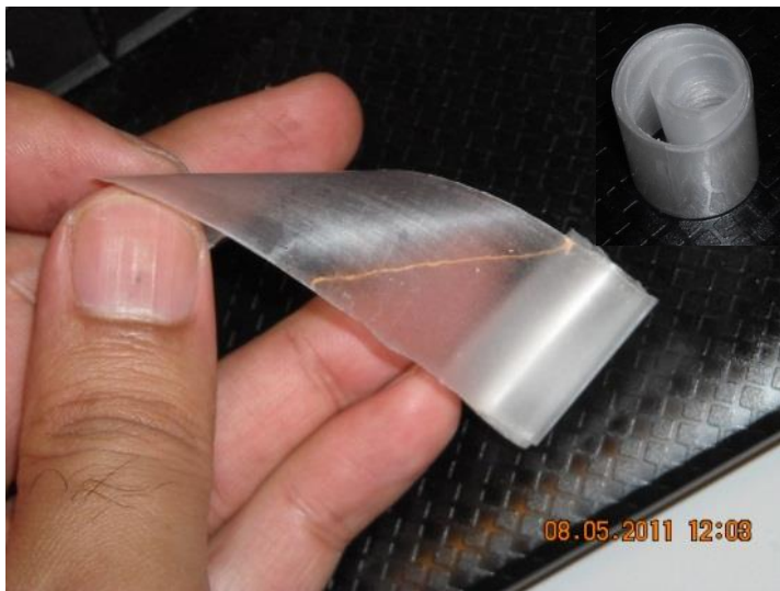
Fig.19. Highly aligned electrospun PS fibers on a thin plastic film
