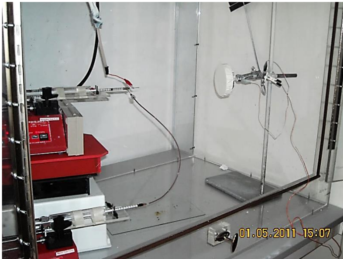
Fig.27. Polystyrene-Polyimide composite fiber spinning
