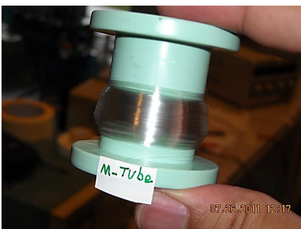
Fig.43 A. Polystyrene microtubes collected on take up wheel
