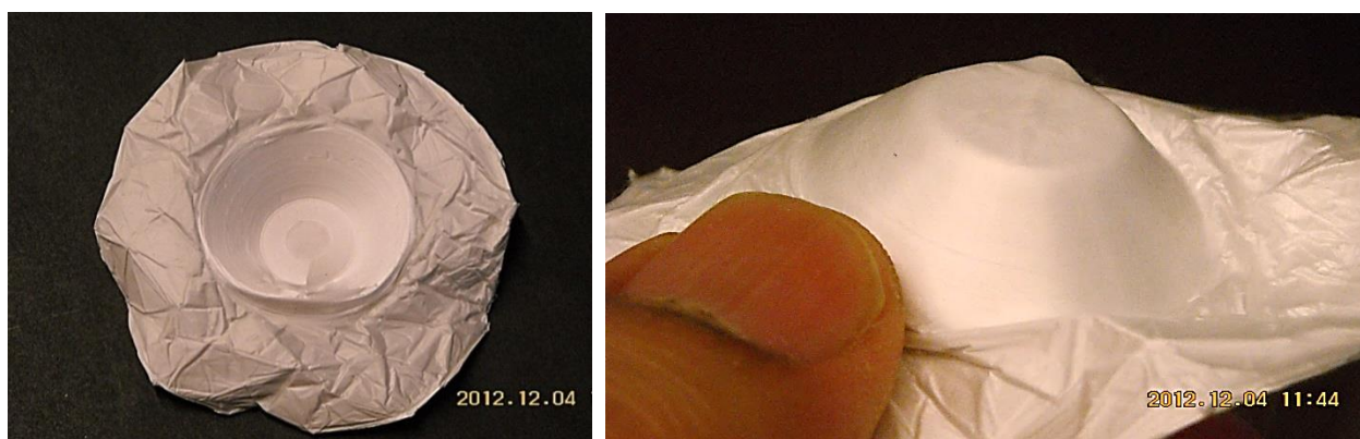
Fig.39 A. Sample 3D scaffold of concentric PLLA fibers produced by spinning on a rotating mold
