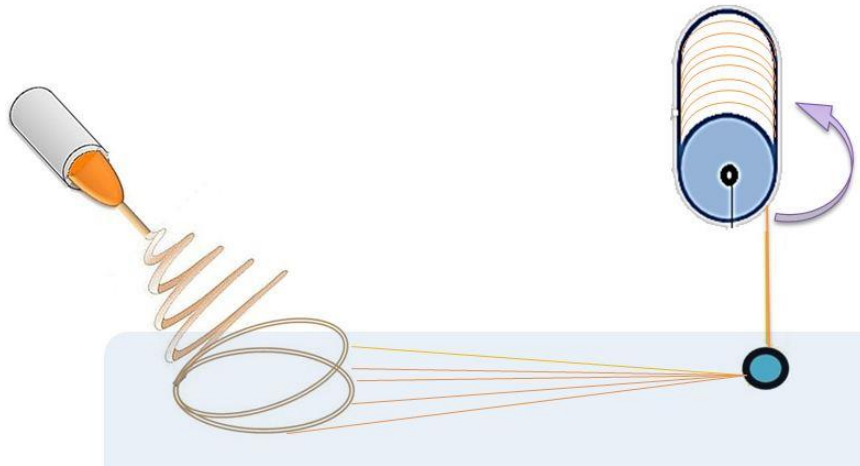
Fig.24. Fibers are spinning randomly on the surface of water while being pulled by a small pulley on the surface of the water. Fibers become aligned during their movement towards the small pulley. Aligned fibers are collected by a Take up Wheel. (Technical details are not shown)
