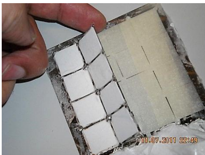
Fig.11. Randomly oriented Poly-L-Lactide Acid fibers accumulated on conductive coverslips
