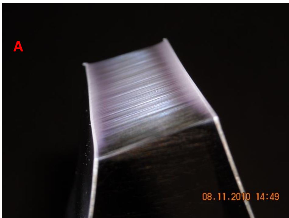
Fig.16. Aligned fibers using gap method
