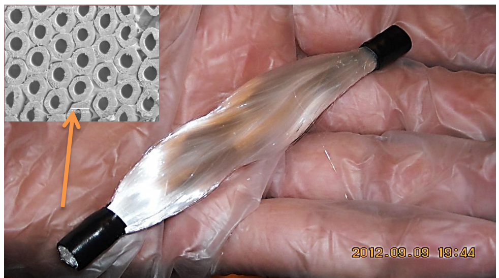
Fig.46. Polystyrene microtube assembly, The tubes in the two ends of the assembly are connected together with Polydimethylsiloxane (PDMS). Inset (SEM image) shows a cross sectional view of one end of the assembly.
