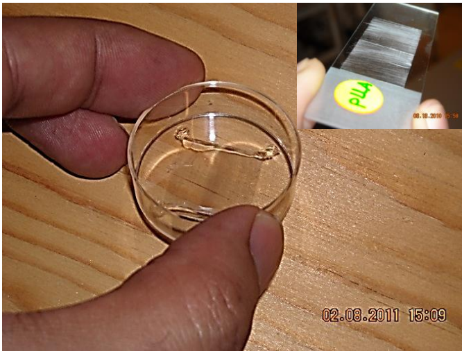
Fig.53: Parallel PLLA fibers ready for culturing
