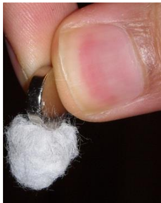
Fig.34. “PS+Iron oxide nanoparticle” composite fibers attracted by a magnet
