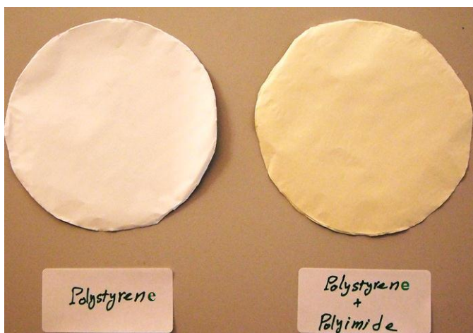
Fig.31. Polystyrene + Polyimide composite fibers spun on aluminum foil
