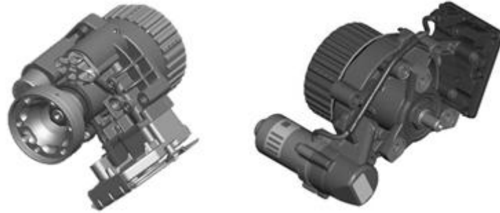
Figure 4.1. A Gen4 (left) and Gen5 (right) coupling. (BorgWarner Inc., 2013)
