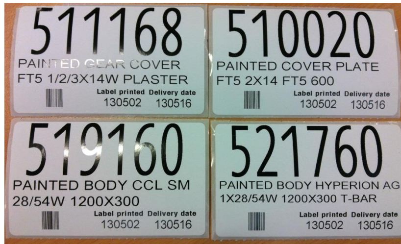
Figure 7.6 Design of printed labels which will travel with WIP. Dimension of one label is 105x63 mm
