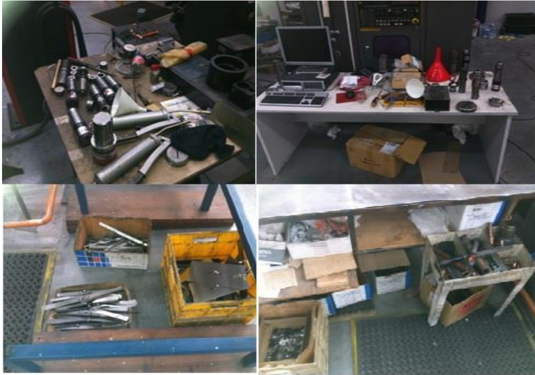
Figure 4.4 Some worst case examples how tools and jigs are stored in the metal shop
